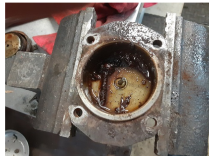
caliper piston assembly from a 1967 E-Type that was in storage for fifteen years.
